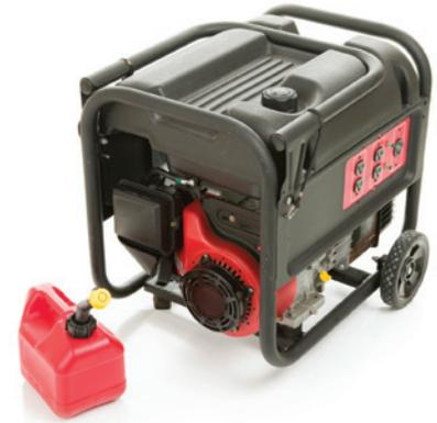
areas, in properly labeled containers, and away from fuel-burning appliances. Before refueling, always turn the generator off and let it cool down.
